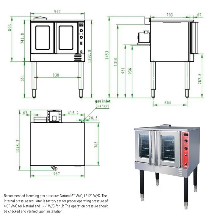
REAR WALL CLEARANCE FROM BACK OF MOTOR: TWO INCHES (2") MINIMUM. SIDE CLEARANCE: 6" SIDE BOTH SIDES FROM COMBUSTIBLE WALLS.
